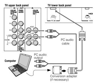
To use a PC, set the monitor output resolution on the PC before connecting it to the TV. The following signals can be displayed:
